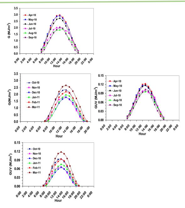
Fig 28: Diurnal variation of monthly means of broadband global radiation flux (G) and global UV radiation flux (GUV), during April 2010 to March 2011 at Delhi.
