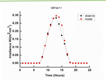
Fig 25: A comparison of total UV flux derived from TUV model and observation
