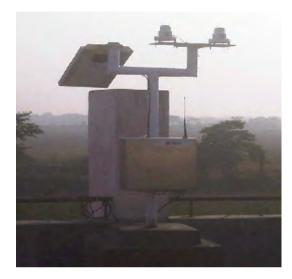
Fig 2: UVB (280-315nm) and UVA (315-400nm) sensors installed at Regional Meteorological Center, Guwahati.
